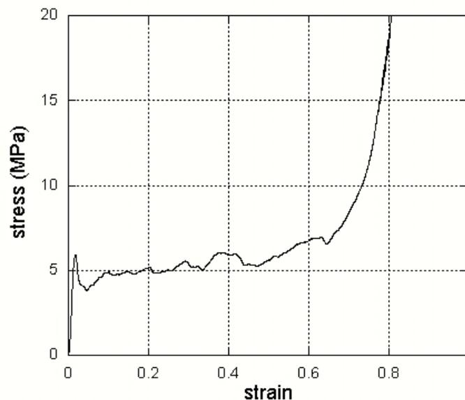
In compression, SAF exhibits a long plateau region in stress over very large strains, meaning it can absorb energy while exerting a constant force. SAF can be produced in a range of densities allowing for the force or energy absorption requirements to be tailored to the application.
